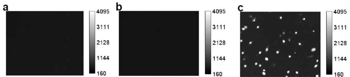
Figure 3.6 Integration of oxygen sensor and fluorescent cell stains. Representative fluorescent image of blank PDMS films showed minimal background emission (a). The PtTFPP sensor without cells showed an emission that was homogeneous in intensity throughout the field of view (b). On the same sensor formulation, dead cells (NIH 3T3 fibroblasts) stained with ethidium homodimer generated local bright spots that were clearly visible over the PtTFPP emission (c) even though the emission wavelengths of the film and stain overlapped.
